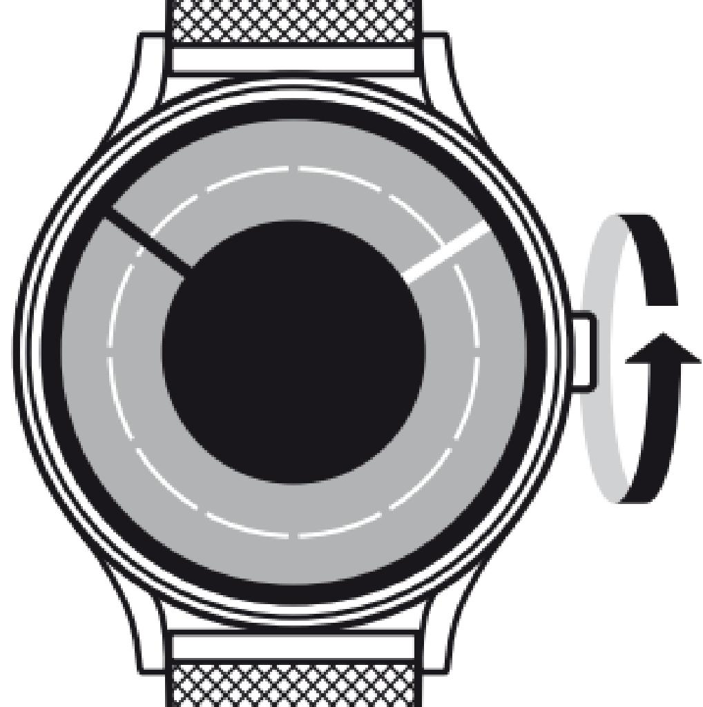
**2** Turn the crown until you reach the correct time. Please note: The crown is always positioned at the 3 AM/PM hour position.
