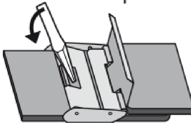
**2** Place a small tool like a screwdriver in the slot to lift the bar according to the image.
